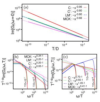
FIG. 4. (a) Temperature dependency of  $\operatorname{Im}[G_f(\omega=0)]$  and the power-law fitting at different fixed points. (b), (c)  $\omega/T$ -scaling behavior of  $G_f(\omega)$  and  $G_B(\omega)$  with the exponent obtained from scaling ansatz.
