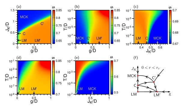
FIG. 12. (a) Boundary entropy  $s(J_K, g, T_0)$  at  $T_0 = 10^{-7}D$  as a function of  $J_k$  and g. (b)  $s(J_K^0, g, T)$  across C' at  $J_k^0 = 0.8D$  vs g and T. (c)  $s(J_K, g = 0, T)$  across C vs  $J_k$  and T. (d)  $s(J_K = 0, g, T)$  near LM' vs g and T. (e)  $s(J_K, g = 0, T)$  near the MCK of r = 0 case vs  $J_k$  and T. (f) Flow diagram for  $0 < r < r_c$  case.
